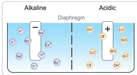
During electrolysis, the cathode has a negative charge and produces alkaline ionized water (pH range 7.5~10) with negatively charged hydroxyl ions, and attracts alkaline minerals - such as calcium, potassium, magnesium, and sodium.
