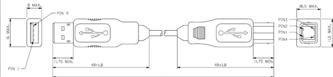
The diagram illustrates the physical dimensions of the CN00214 USB A-B Cable. It shows two views: one for the Type A connector and one for the Type B connector. Key dimensions include:
