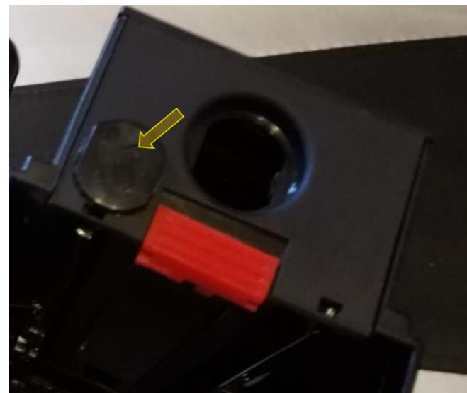
3. Insert Lock and locking cam instead of removed part
