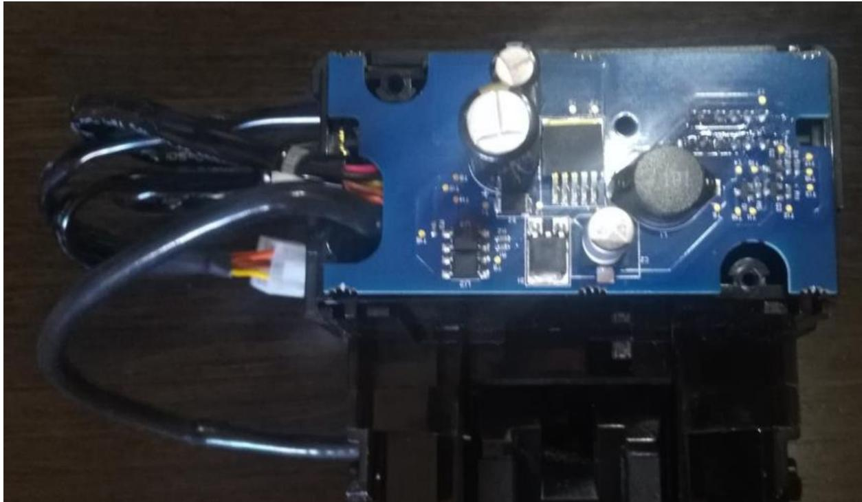
3. Spread the wires and close the cover using 2 screws:
