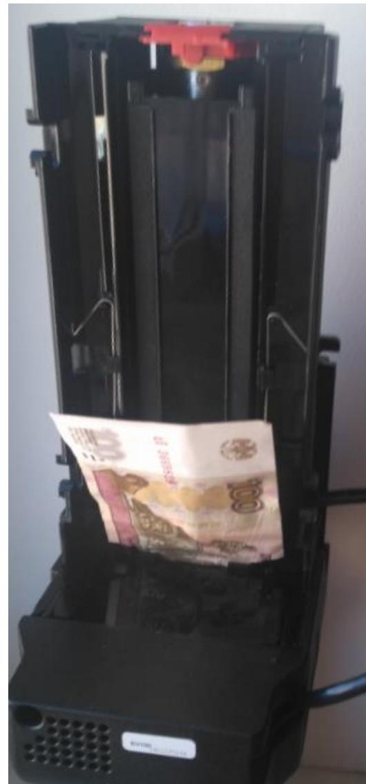
3. Inspect the visible parts of validator for any banknote remains, then attach cashbox. Validator should reinitialize sensors and be ready to work.
