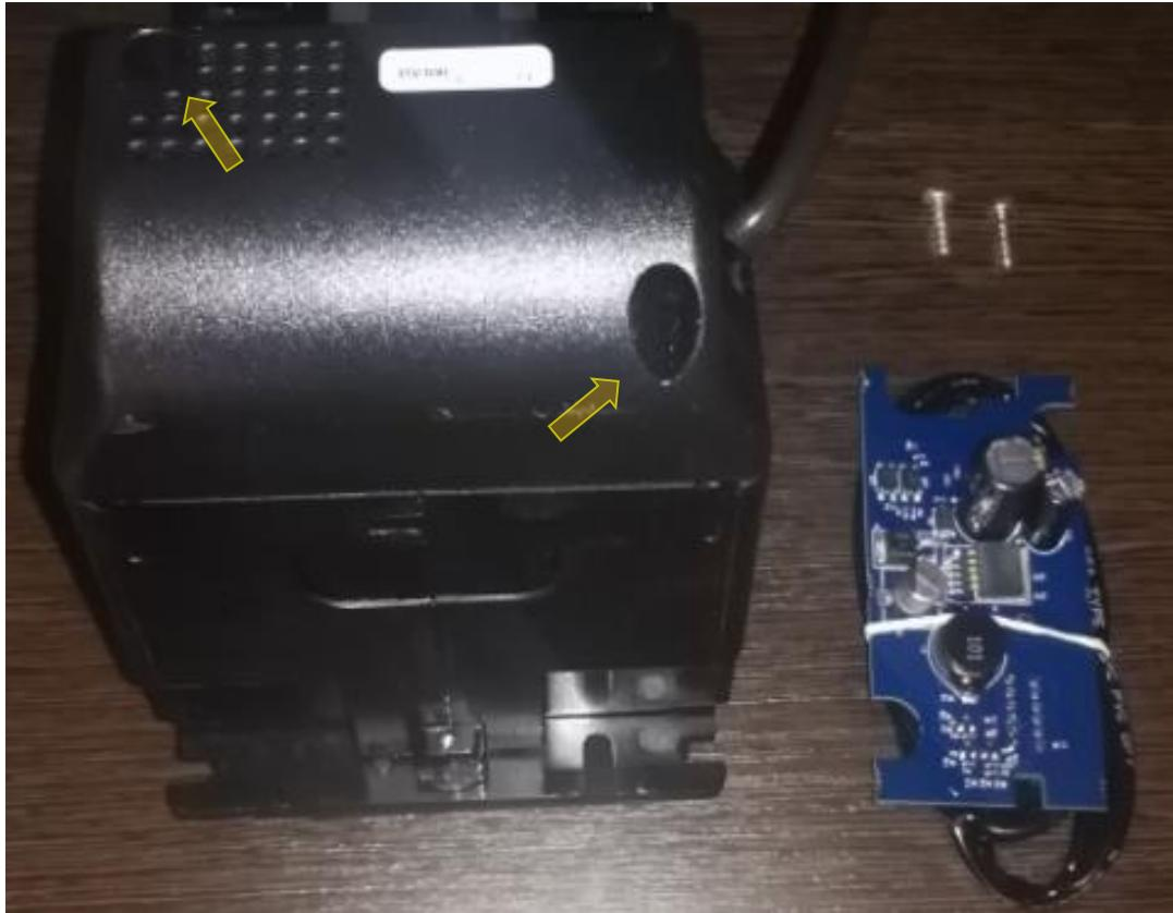
2. Place MDB PSU into BV100 Board MDB slot
