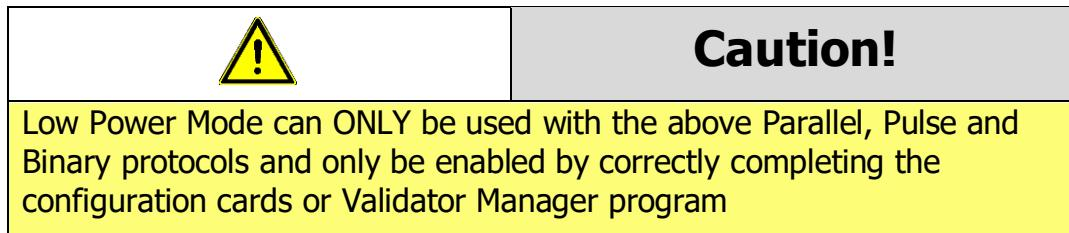
Low power Mode can be used with all none serial communication protocols to reduce the power consumption of the BV100 when idle. When the BV100 is in this state the current consumption is reduced.
