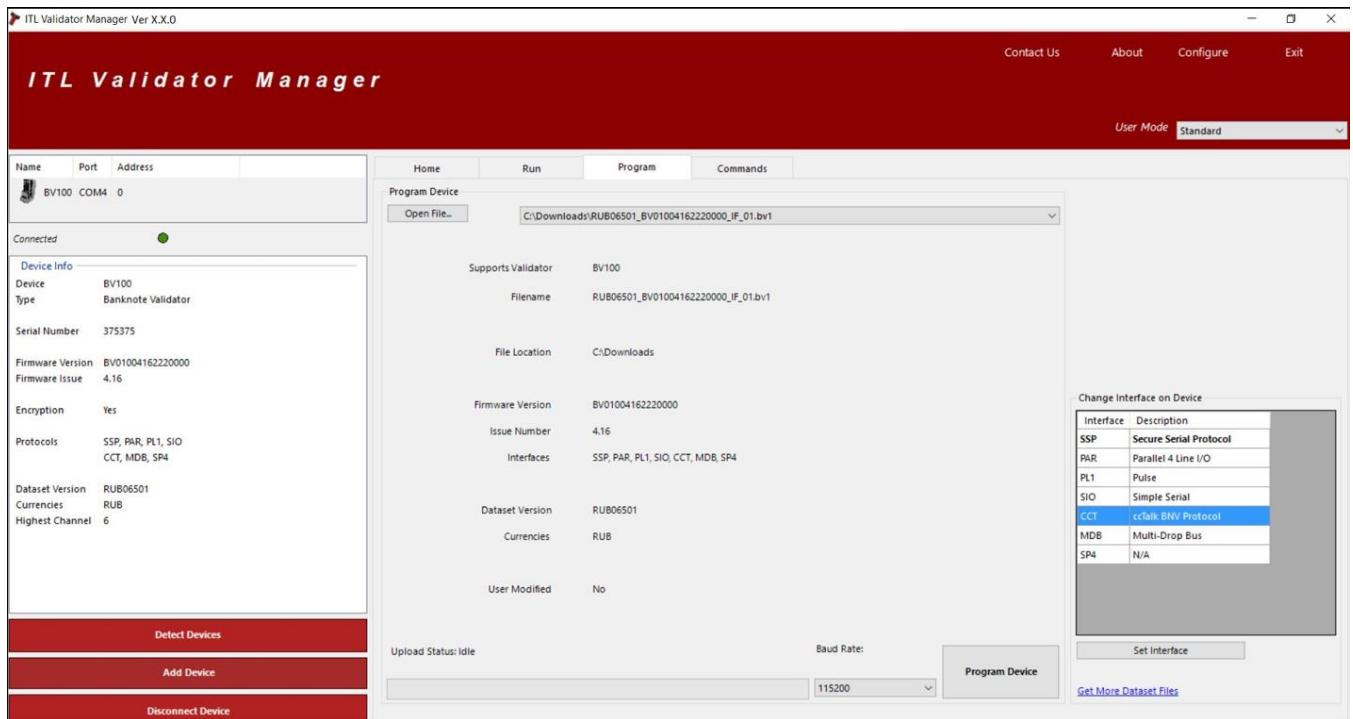
Once the file has been selected its information will be populated and the Program device tab will become active. Finally hit 'Program Device', the unit's bezel will now begin to flash signaling the update has begun. If it's unable to program device, then incorrect file type was chosen.
