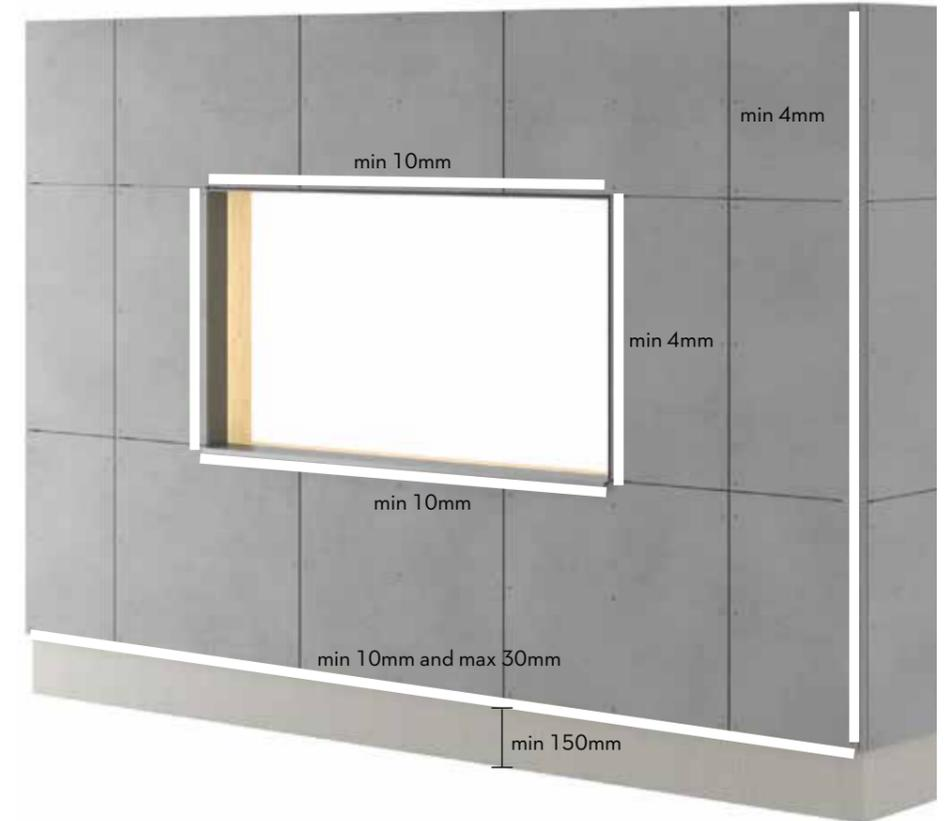
Make sure to follow the guidelines regarding distances described in this manual. The facade board should finish between 10 and 30mm below the bottom end of the substructure. For overhang and similar, the maximum distance is 100mm.
