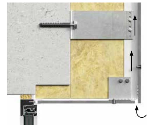
A horizontal free ventilation opening must be maintained above windows and doors as well. This ventilation gap must be at least 10mm wide. If steel, aluminium or plastic perforated profiles are used, a ventilation area opening of minimum 100cm<sup>2</sup> per meter is required. The opening at the base is also used to drain moisture that has entered the facade.
