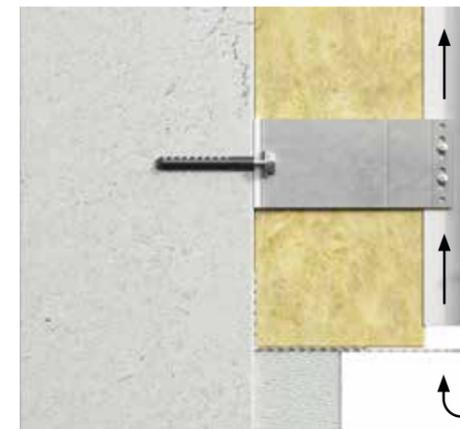
Air is pulled into the construction through an opening at the base of the facade, and it must be ensured that unobstructed ventilation is possible throughout the facade's height. There should be a ventilation gap of minimum 10mm, or equivalent 100cm<sup>2</sup> per meter. If perforated profiles are used, a ventilation area opening of minimum 100cm<sup>2</sup> per meter is required. The opening at the base is also used to drain moisture that has entered the facade.
