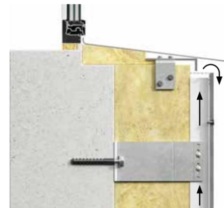
A horizontal ventilation opening of minimum 10mm or equivalent to 100cm<sup>2</sup> per meter should be maintained beneath windows or other openings where a sill is used. This ventilation gap is usually formed between the top edge of the facade boards and the bottom edge of the sill. It is recommended that the sill projects a minimum of 30mm beyond the front of the facade. This ensures that the water running from the sill does not enter the structure.
