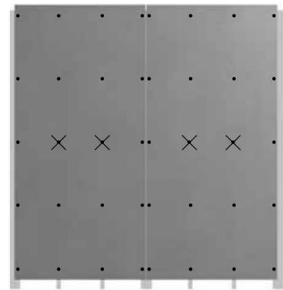
Example: Vertically mounted boards with two intermediate aluminium profile
