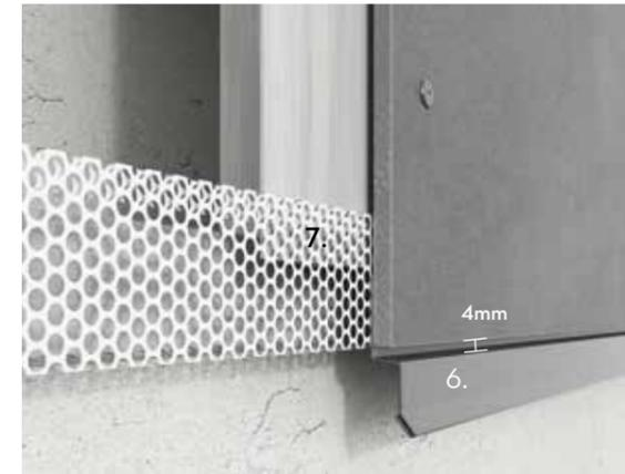
Cembrit Drip Small is used to drain water away from the supporting structure or where neat detailing is required at the foot of the facade. The profile can be used in conjunction with Cembrit Ventilated Profile to ensure that insects and vermin cannot enter the cavity behind the facade boards. There should be a minimum 4mm gap between the board edge and the profile.
