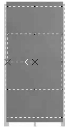
Illustration of correct rivet installation sequence.
