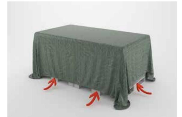
Replace the plastic with a tarpaulin. It is very important that there is ventilation all around the tarpaulin and also on top of the pallet under the tarpaulin. This is done to make sure that condensation is reduced as much as possible.
