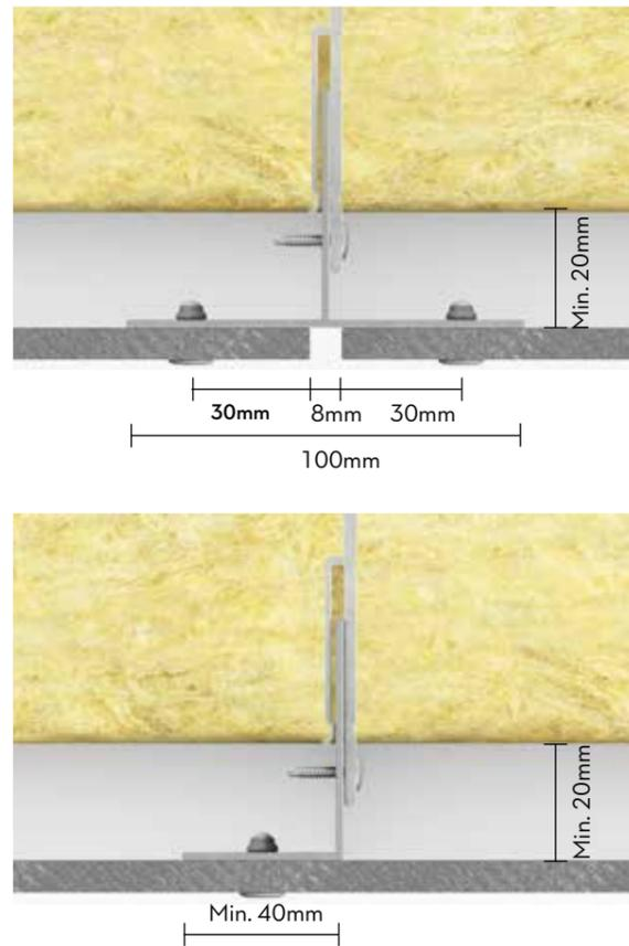
To ensure that boards are able to accommodate movement without damage, please adhere to the following Cembrit guidelines for correct fixing centres and hole sizes.
