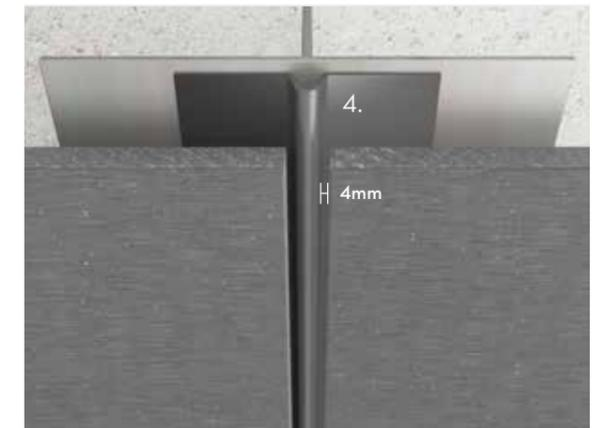
Cembrit Caulking Profile can be used in both vertical and horizontal joints. It is not mandatory to use Cembrit Caulking Profile, but it provides excellent joint solutions. The profile is installed in the same way as Cembrit External Corner. There should be a minimum 4mm gap between the board edge and the Cembrit Caulking Profile.
