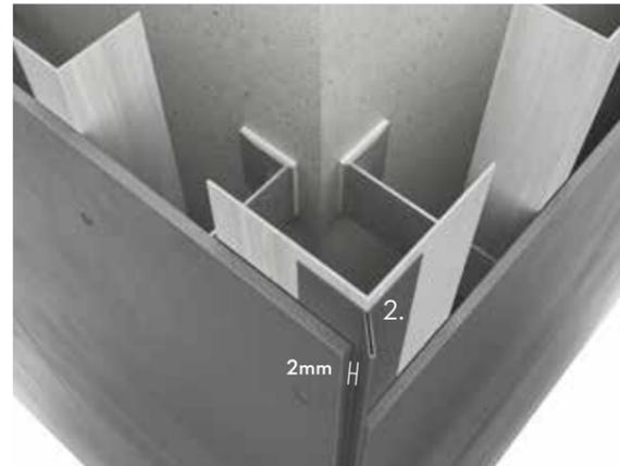
Cembrit External Corner Peak can also be used for 90° external corner constructions. It is installed in the same way as Cembrit External Corner Small. The distance from the inside edge of the facade boards to the profile should be a minimum of 2mm.
