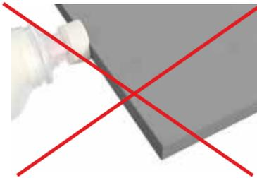
All cut edges (except Cembrit Patina) must be sealed with Cembrit Edge Sealer to ensure protection of the cut edges. Use the Cembrit Edge Sealer Set with Applicator and Sponge. Avoid getting Edge Sealer liquid on board faces. If this does occur, remove any liquid with a lint-free cloth immediately.
