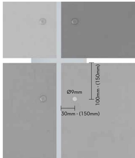
Example of vertical substructure
