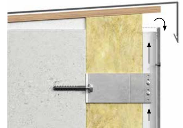
The passage of air must be maintained at the top of the facade whether it abuts to a roof or other structure. Just as at the base, there must be a ventilation gap of a minimum of 10mm or 100cm<sup>2</sup> per meter.
