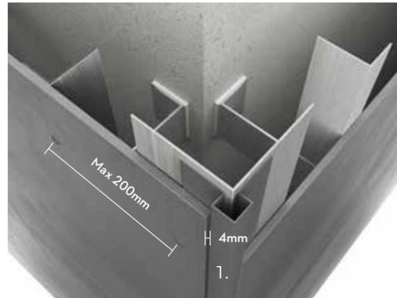
Cembrit External Corner Small is used for 90° external corner constructions, to create a securely finished detail. Use double sided tape to temporarily fix the profile to the facade board before fixing it with rivets. Make sure the correct edge distances and hole sizes are used. The distance from the corner edge to the wall T or L profile should not exceed 200mm. There should be a minimum 4mm gap between the board edge and the profile.
