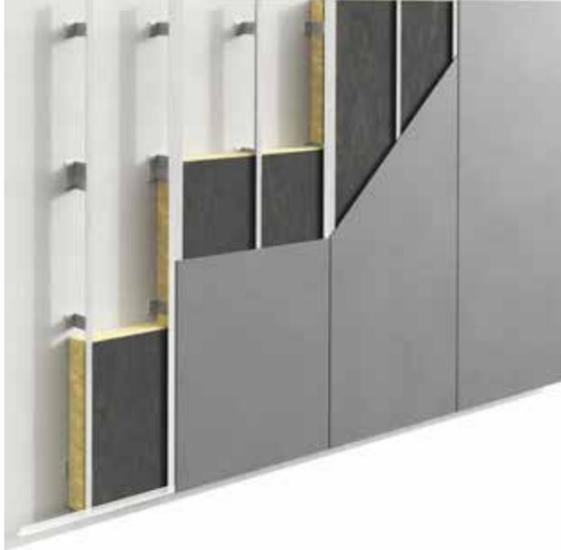
Cembrit facade boards can be mounted on many different types of support systems. This manual deals with the installation of Cembrit facade boards on an aluminium system. Typically, an aluminium system for fibre cement consists of 'T' profiles at the joints and L profiles as centre profiles. These are vertically mounted on the load-bearing wall using brackets. Insulation is mounted between the profiles on the load-bearing wall. This is the system shown in this installation manual.
