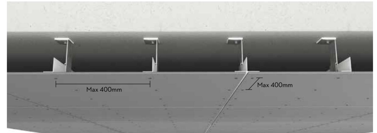
When using Cembrit facade boards as ceiling or soffit, you can normally use a regular aluminium system with brackets and T and L profiles, but for larger cavities, you need to contact an aluminium manufacturer to make sure the system fits your needs. The number of brackets and types of anchoring used for the type of deck/ceiling has to be calculated, and the manufacturer's instructions should always be followed.
