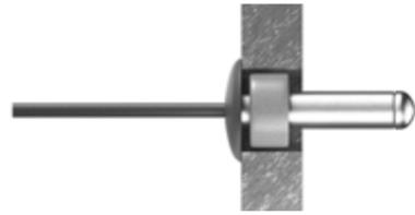
X : Fixing position hole diameter Ø9 mm.
