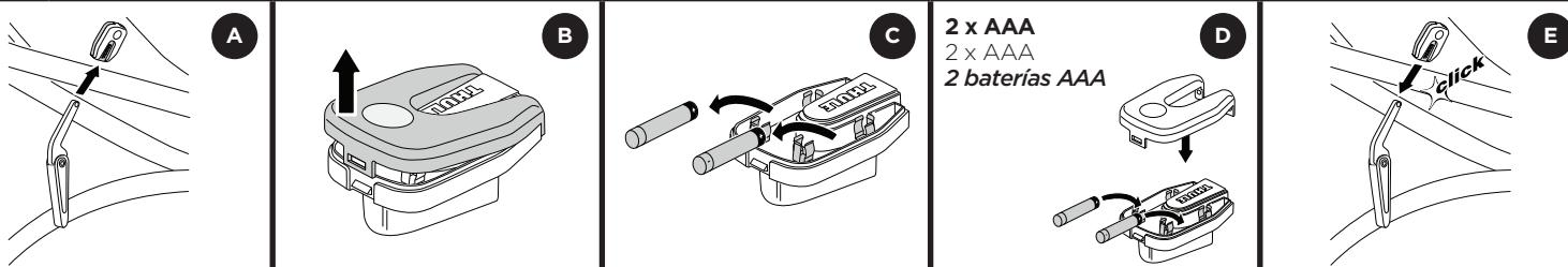
**NOTE:** AAA Lithium or Alkaline batteries are preferred. Rechargeable batteries are compatible with the light but may lose their charge quickly.
