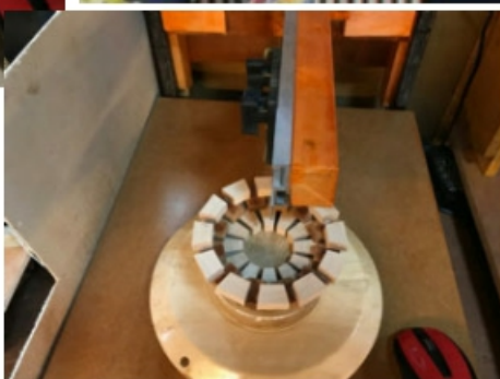
Above & Right: These two pictures show Johns vertical jig for building up open segmented work
