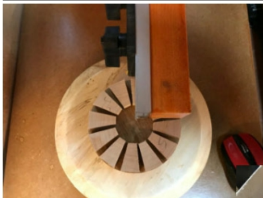
Above & Right: These two pictures show Johns vertical jig for building up open segmented work
