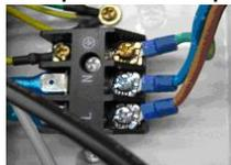
**Figure 9: Mains connection terminals.**
