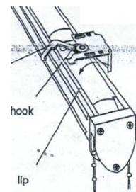
To attach blind to the brackets you have just fitted simply raise the headrail into position as illustrated.
