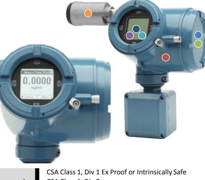
Approvals Application Restrictions CSA Class 1, Div 1 Ex Proof or Intrinsically Safe CSA Class 1, Div 2 ATEX and IECEx are also available Continuous Multiphase Density/Viscosity Limit: 1.4 g/cc / 500 centipoise High Velocity Gas Limit: 0.2 Mach
