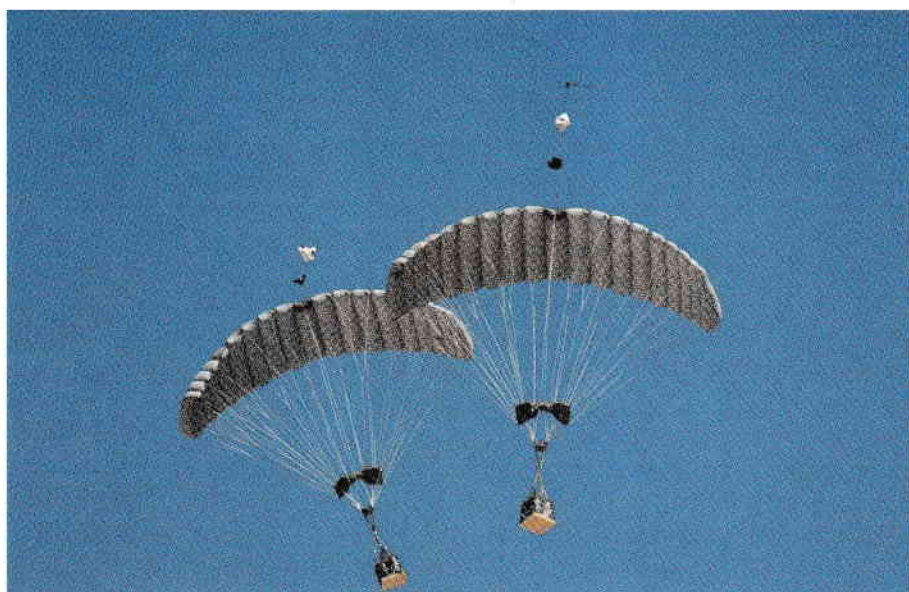
Colis autoguidé en vol Self-guided package in flight
