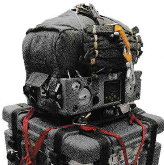
Colis autoguidé prêt au largage Self-guided package ready for airdropping
