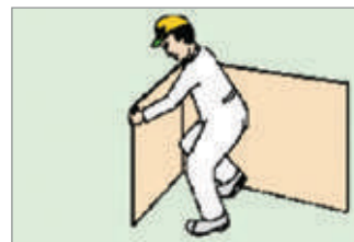
Snap Siniat Plasterboard and cut other side of paper
