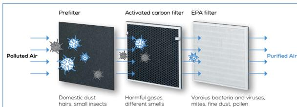
Function principle of the air purifier: Domestic dust, animal hairs, smells, pollen, harmful gases and various bacteria and viruses are filtered out of the air using a triple-layer filter system.
