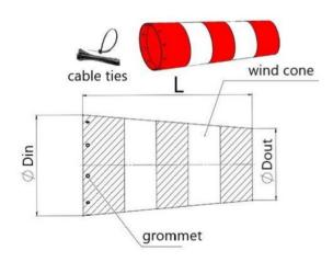
Cone which has the shape of a truncated cone and can be sewed from various fabrics.
