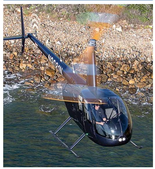
Four-seat R44 Raven I and Clipper I helicopters are high performing, reliable and easy to maintain. R44s have a two-bladed rotor system, T-bar cyclic, streamlined instrument panels, and a crashworthy fuel system.
