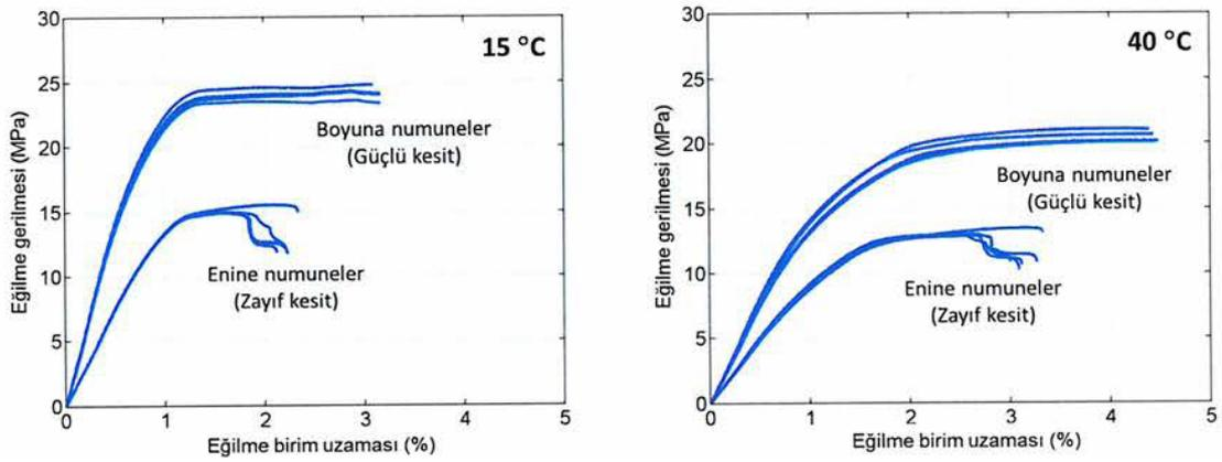
**Figure 6.** Stress-unit strain diagrams obtained from bending tests
