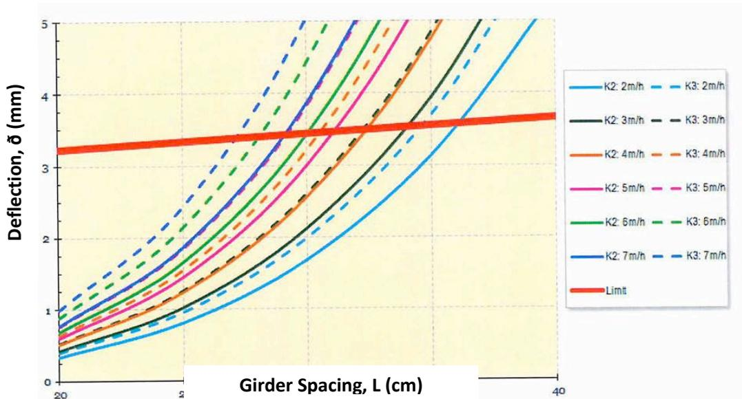
Figure E. Deflection diagrams for EKOPLAK strong section in multi span vertical application
