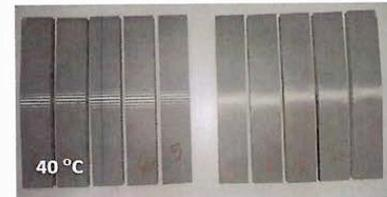
**Figure 5.** Longitudinal and transversal specimens during bending tests at 15°C and 40°C
