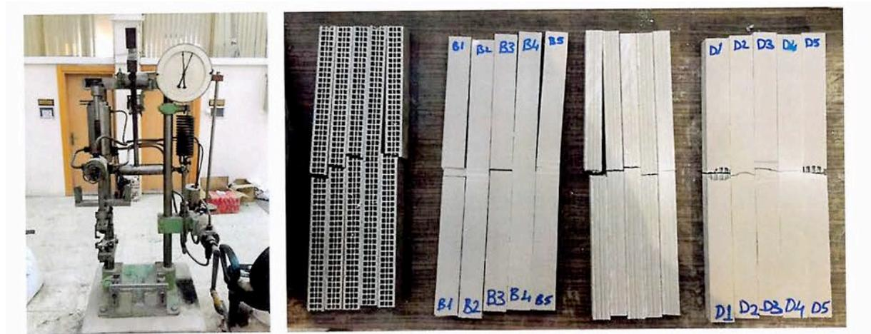
**Figure 7.** Charpy impact test apparatus and sample sets
