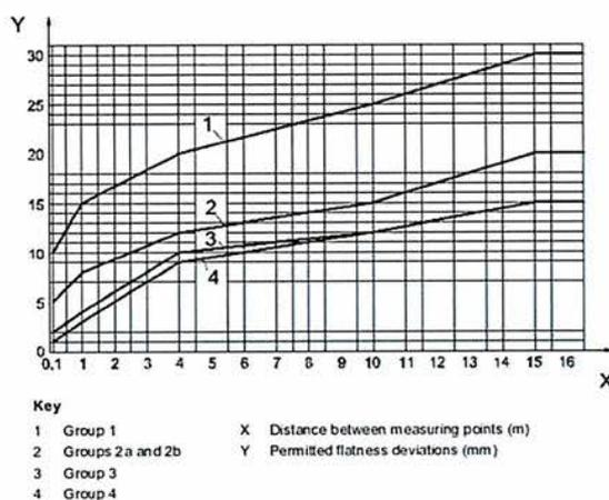
Figure 5 — Permitted flatness deviations for upper surfaces of floors and screed (groups from Table 3)
