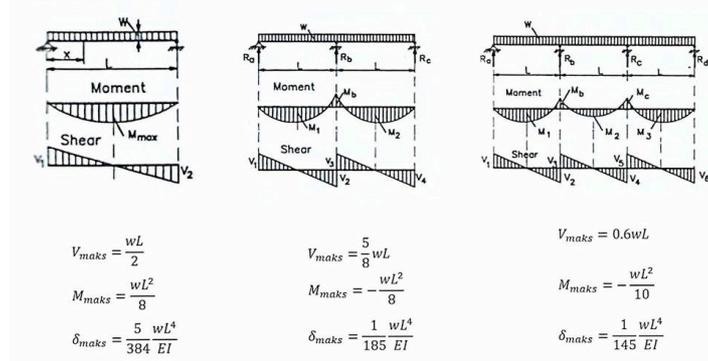
**Figure 11.** Maximum shear, torque and deflection values for single span and multispan beams
