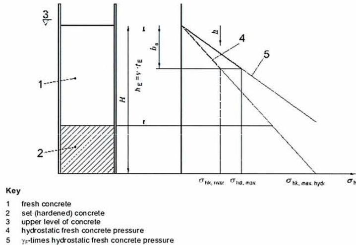
**Figure 10.** Fresh concrete pressure-vertical formwork height diagram (DIN 18218:2010-01)
