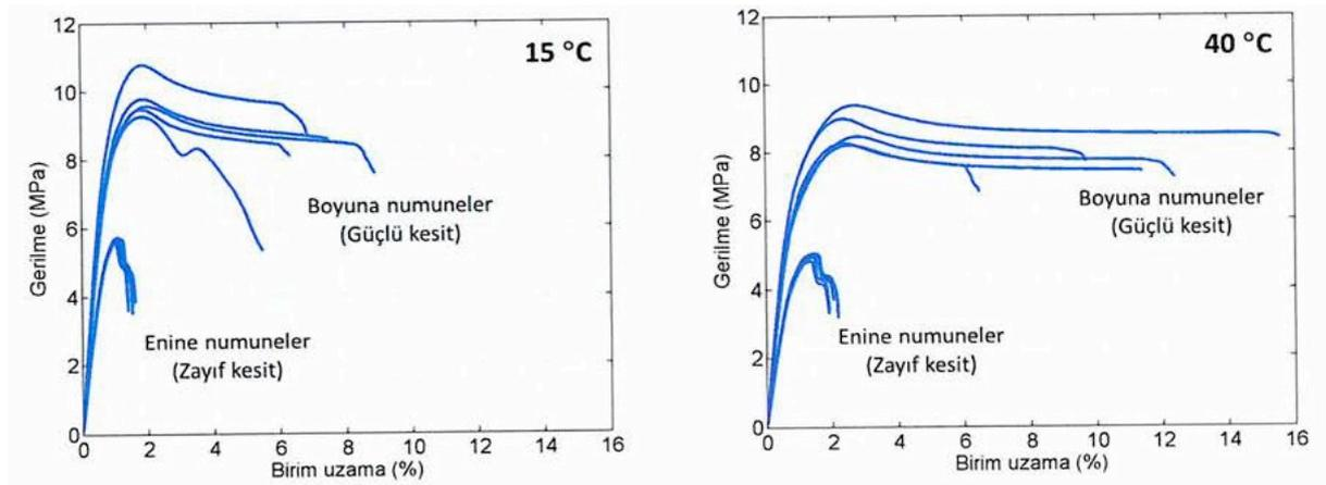
Figure 4. Stress-unit strain diagrams obtained from tension tests
