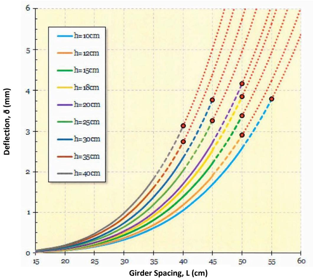
Figure A. Deflection diagrams for EKOPLAK strong section in single span application
