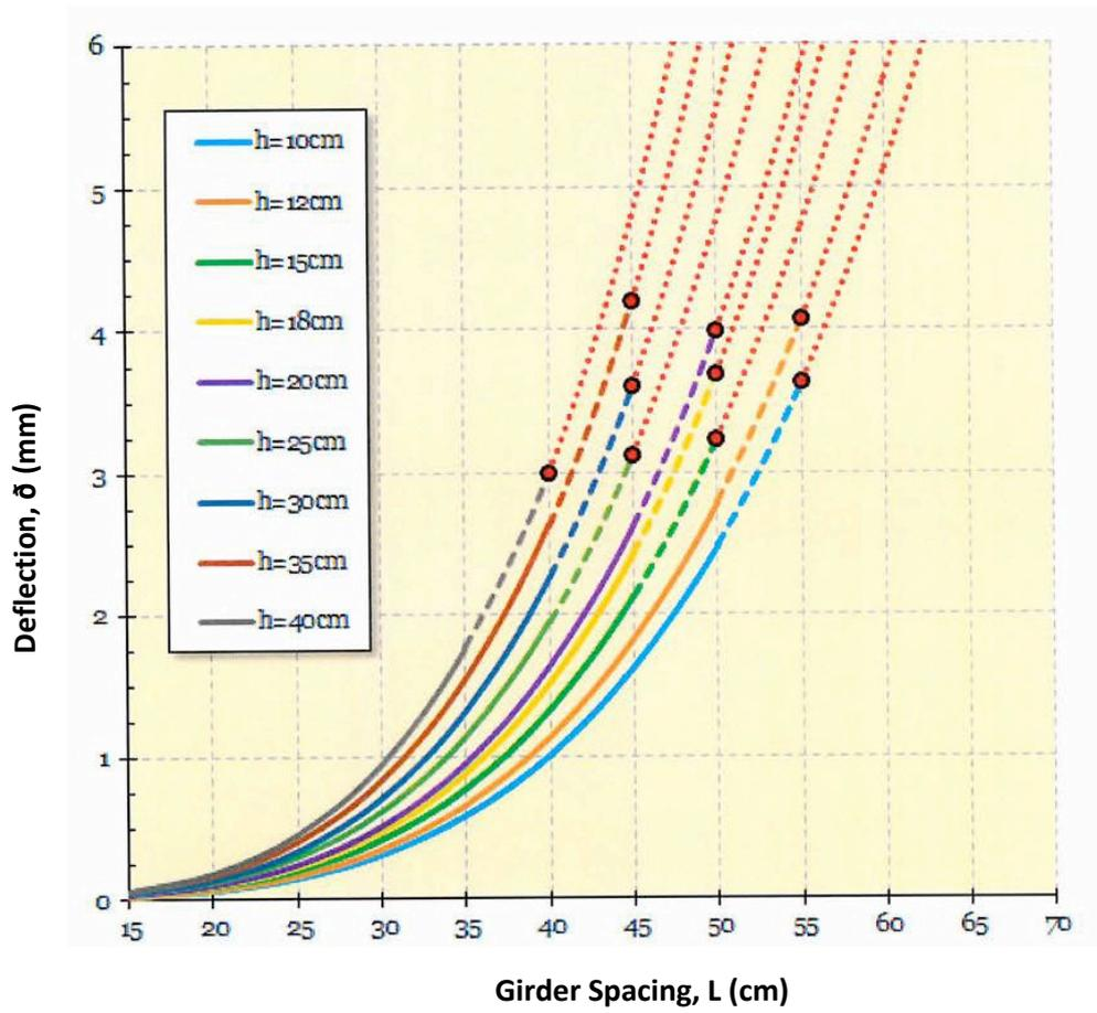
**Figure D.** Deflection diagrams for EKOPLAK weak section in multi span application
