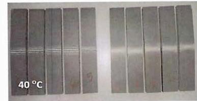
**Figure 5.** Longitudinal and transversal specimens during bending tests at 15°C and 40°C
