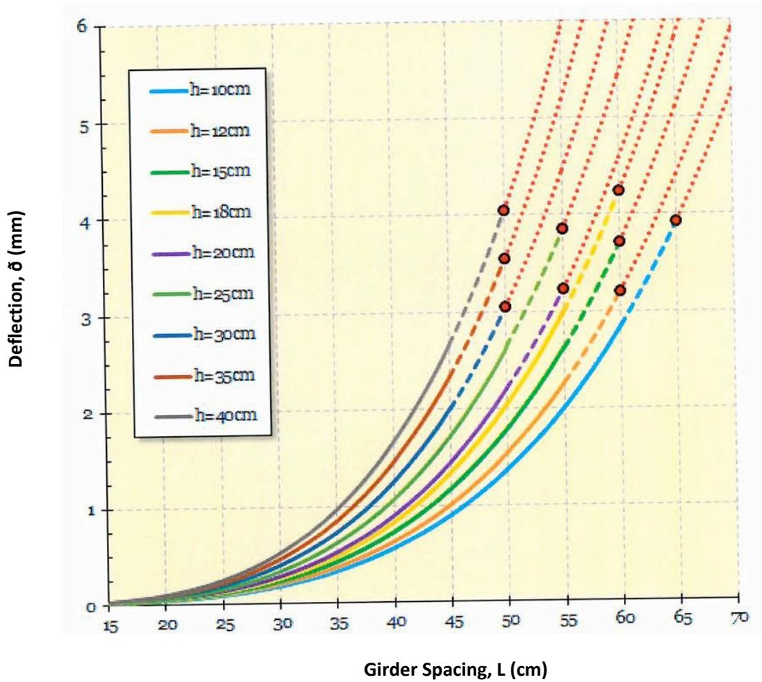
Figure C. Deflection diagrams for EKOPLAK strong section in multi span application
