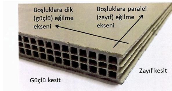
**Figure 1.** EKOPLAK polypropylene hollow board cross section
