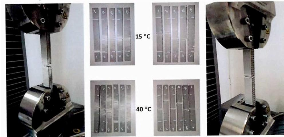
Figure 3. Longitudinal and transversal specimens during tension tests at 15°C and 40°C
