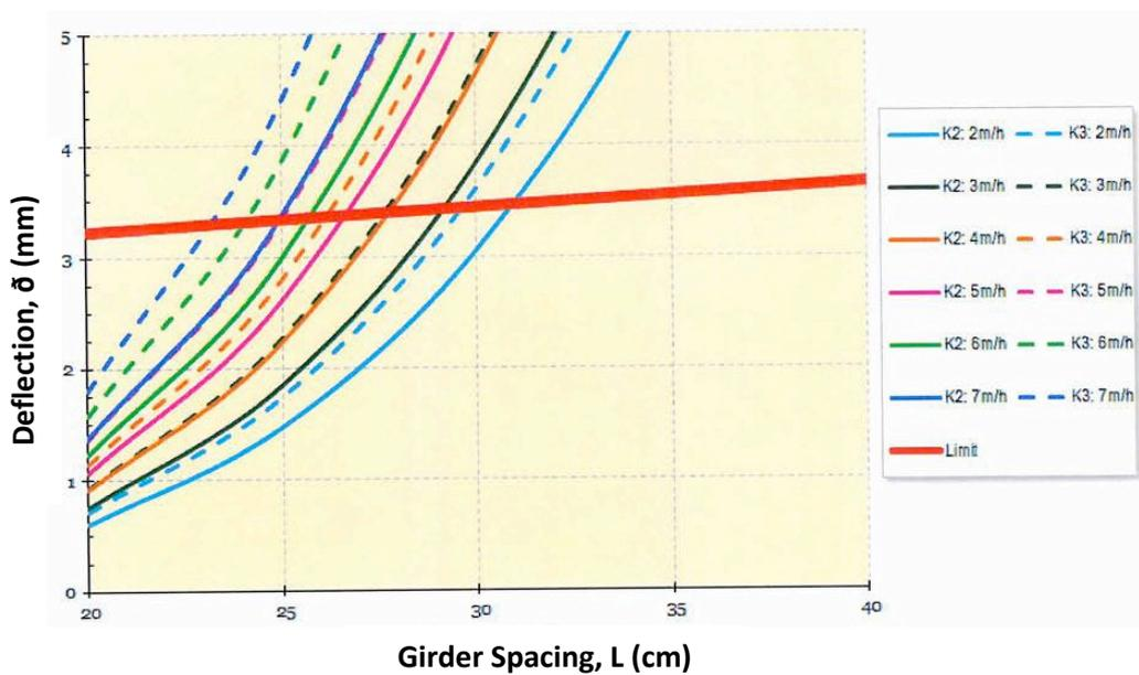
Figure F. Deflection diagrams for EKOPLAK weak section in multi span vertical application
