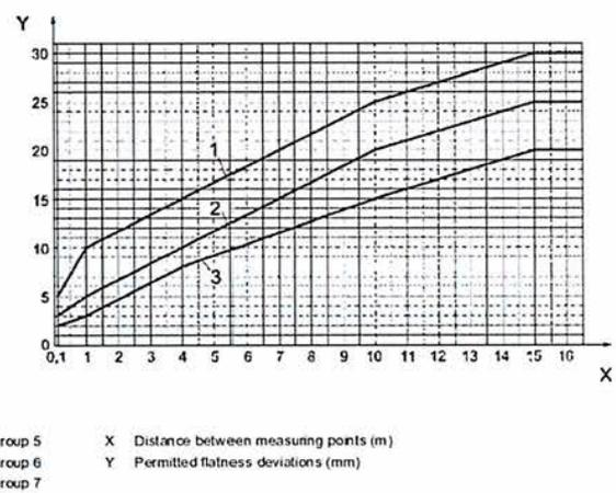
Figure 6 — Permitted flatness deviations for wall surfaces and soffits (groups from Table 3)
