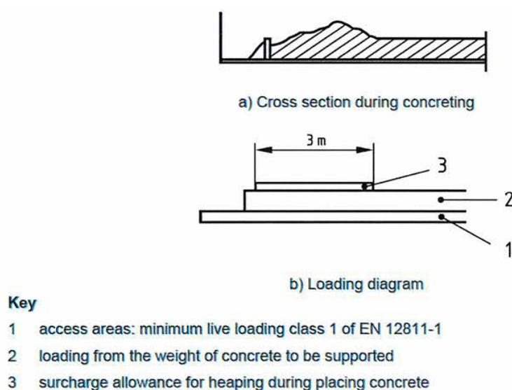
**Figure 9. Design loads considered in fresh concrete casting (EN 12812:2008)**
