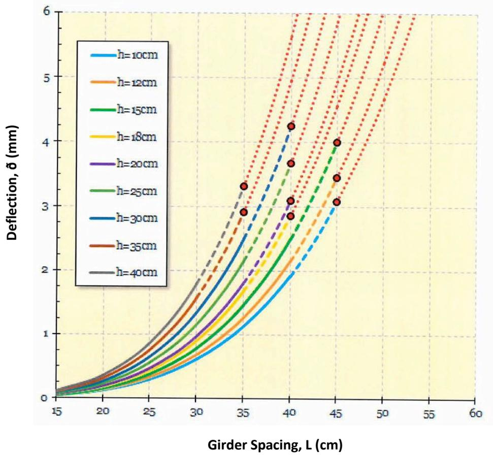
Figure B. Deflection diagrams for EKOPLAK weak section in single span application
