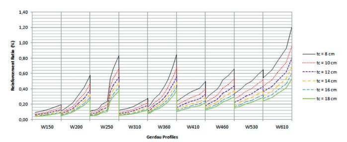
**Figure 10**Reinforcement ratio x analyzed Gerdau profile
