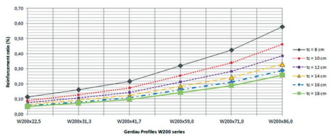
**Figure 9**Reinforcement ratio x analyzed Gerdau profile, W200 series
