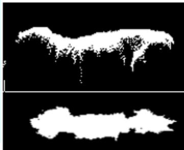
Figure.13. The actual X-Y-Z axis point cloud is converted through projection towards X-Z (above) and the X-Y projection result (below)
