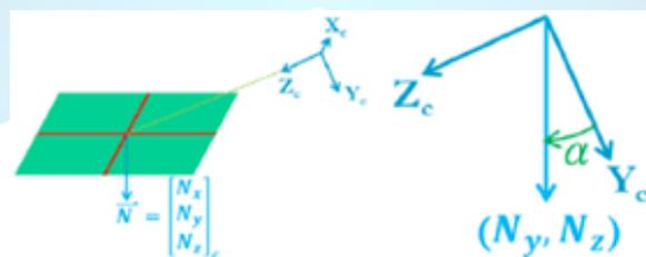
Figure.6. Relationship between the alpha value of the transformation matrix and the plane normal vector
